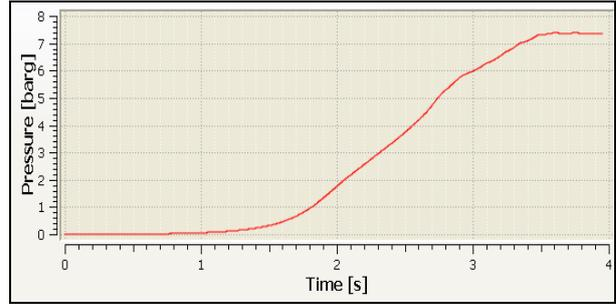
Figure 6 DESC simulation of Icing Sugar explosion in a 400-m<sup>3</sup> cylindrical silo without explosion vents.
