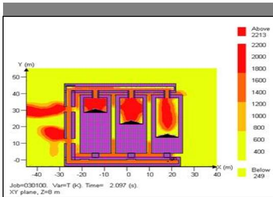
Figure 11. 2D cut-plane images of the Imperial Sugar silo simulation show temperature developments at 2.097 s.
