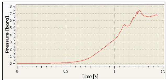
Figure 15, Pressure-time curves of a (-200 mesh) PE silo explosion (The safety explosion doors disabled)
