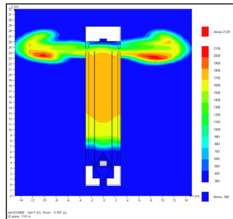
Figure 16. 2D cut-plane (X-Z) image shows temperature development of PE explosion.
