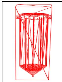
Figure 13. 3D CAD image of polyethylene silo (wireframe style).
