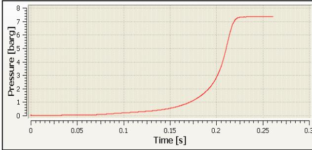
Figure 2 DESC simulation of Icing Sugar explosion in a 20-L spherical chamber.
