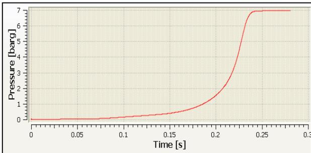
Figure 4 DESC simulation of Granulated Sugar explosion in a 20-L spherical chamber.
