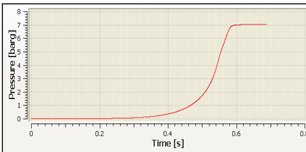
Figure 5 DESC simulation of Granulated Sugar explosion in a 1-m<sup>3</sup> spherical chamber.
