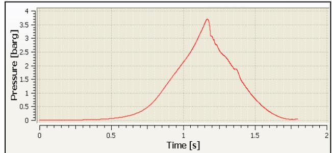
Figure 14. Pressure-time curves of a (-200 mesh) PE silo explosion (the safety explosion doors enabled).
