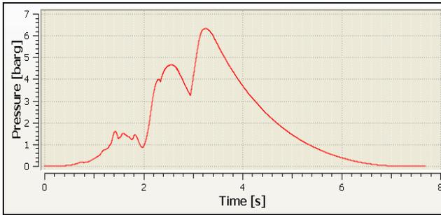
Figure 9 DESC simulation of Icing Sugar explosion in a 3700-m<sup>3</sup> Imperial Sugar Silos geometry with explosion vents (PP 2 bar).
