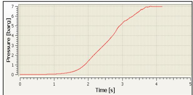
Figure 7 DESC simulation of Granulated Sugar explosion in a 400-m<sup>3</sup> cylindrical silo without explosion vents.
