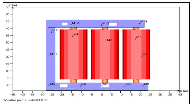
Figure 8 DESC representation of interconnected 3700-m<sup>3</sup> silos.
