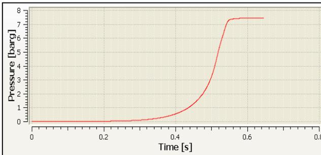
Figure 3 DESC simulation of Icing Sugar explosion in a 1-m<sup>3</sup> spherical chamber.
