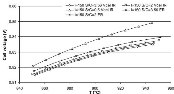
Figure 2: Effect of steam-carbon ratio on the cell voltage at I=150 mA/cm<sup>2</sup>.
