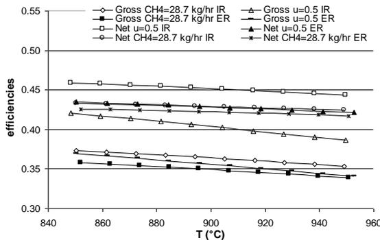
Figure 7. Efficiencies of the cycles at  $I=107$  mA/cm<sup>2</sup>,  $u=0.5$  and CH<sub>4</sub> flow rate=28.7
