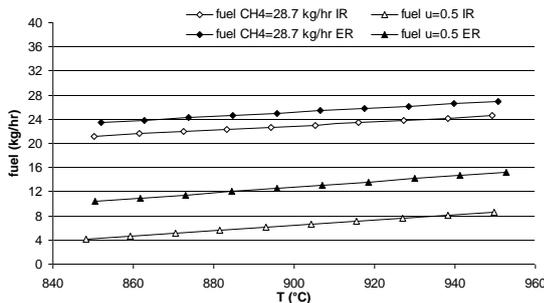
Figure 6. Mass flow rate of fuel as a function of operating temperature at  $I=107$  mA/cm<sup>2</sup>.
