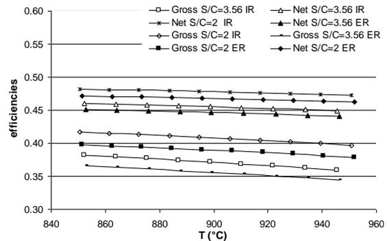
Figure 4. Effect of steam-carbon ratio on the efficiencies at I=150 mA/cm<sup>2</sup>.
