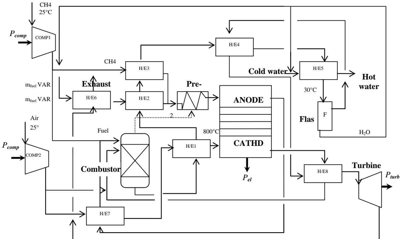
Figure 1: Schematic diagram of internal reformed SOFC system (COMP: compressor; H/E: heat exchanger).
