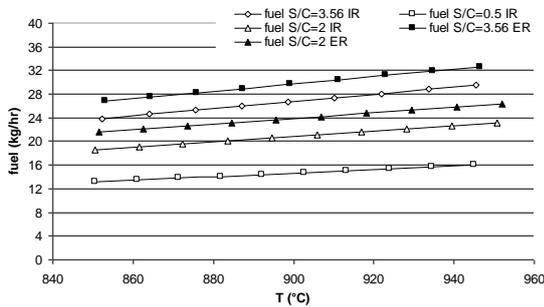
Figure 5. Effect of steam-carbon ratio on the fuel flow rate at  $I=150$  mA/cm<sup>2</sup>.
