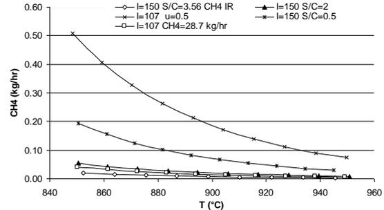
Figure 3. The mass flow rate of remaining CH<sub>4</sub> in the anode exit.
