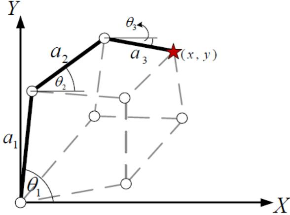
Figure 1 3DoF of robotic arm. Different possible solution to approach point  $(x, y)$
