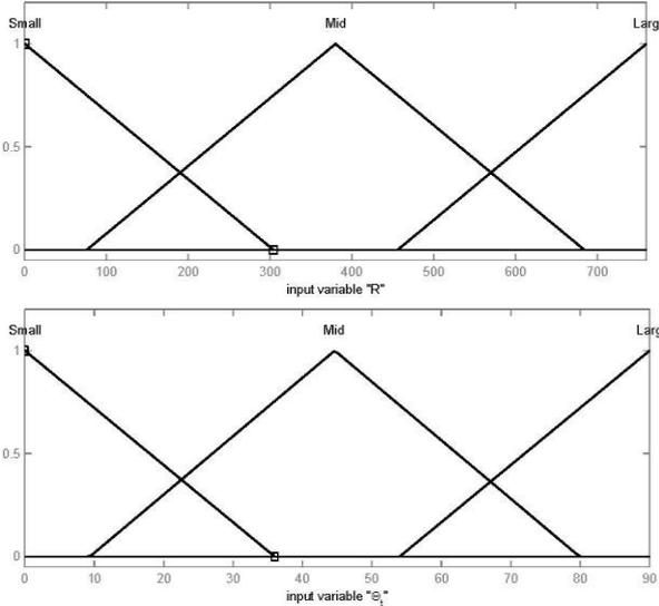
Figure 3 FIS membership functions for input variables: R and  $\theta_t$ .
