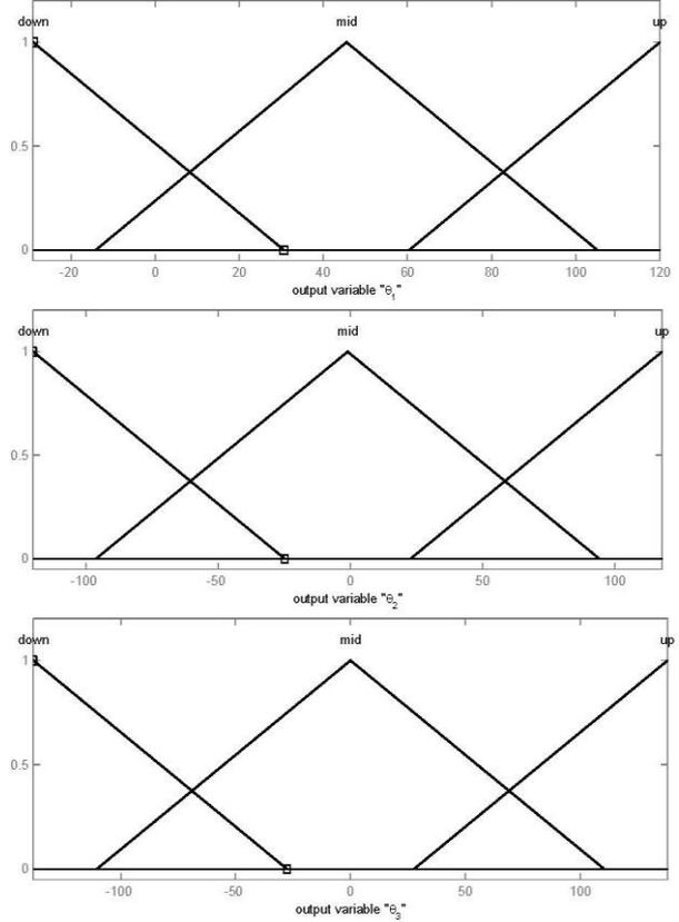
Figure 4 FIS membership functions for output variables:  $\theta_i, i \in \{1,2,3\}$
