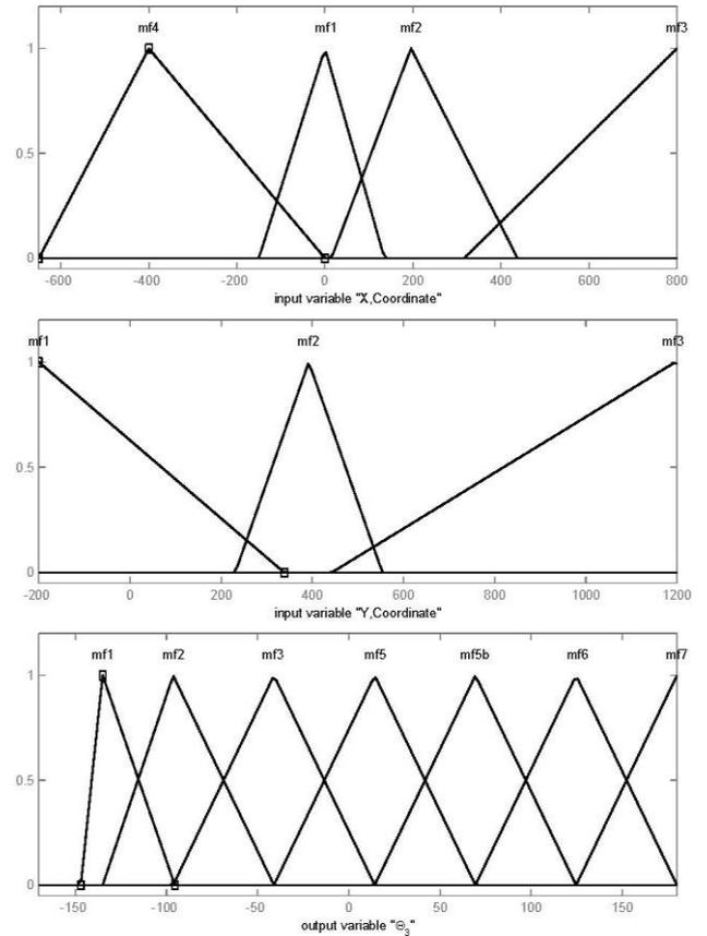
Figure 2 FIS membership functions for input variables:  $x$  and  $y$ , and output variable  $\theta_3$ .
