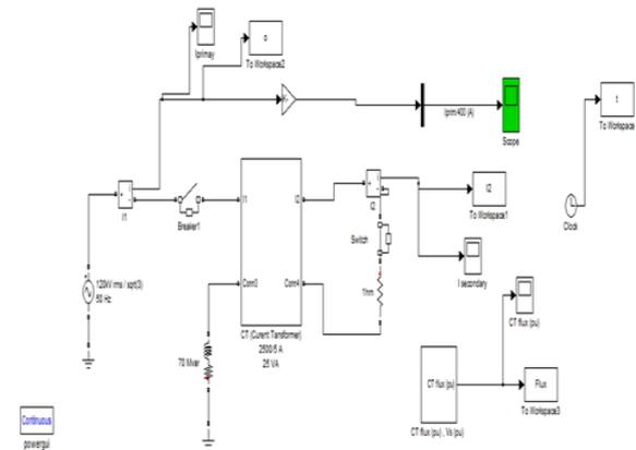
Figure 6 The Circuit Used In MATLAB Simulink of CT
