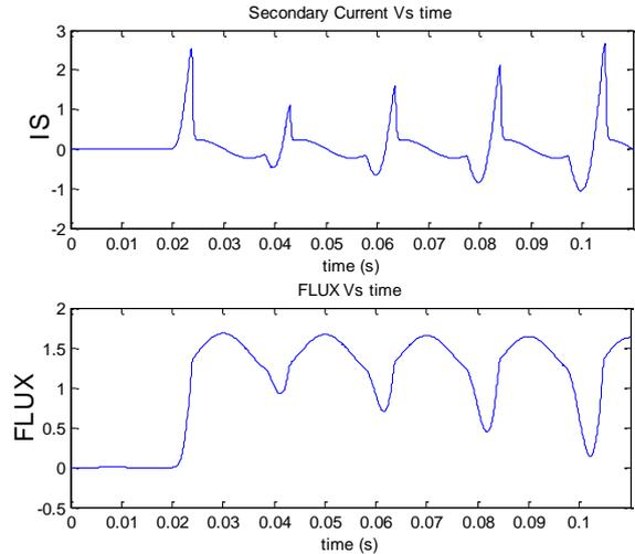
Figure (10) Simulink Output with Hysteresis For Secondary Current and Flux.
