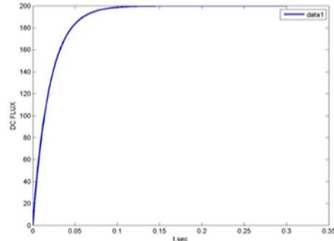
Figure 5 Dc Flux in the CT core
