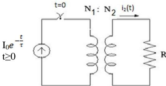
Figure 4 CT excited by The Dc Offset Current Source
