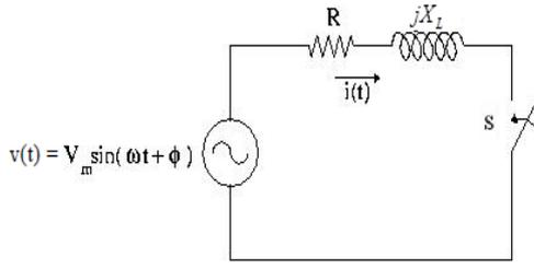
Figure 2 Transmission Line with Voltage Source
