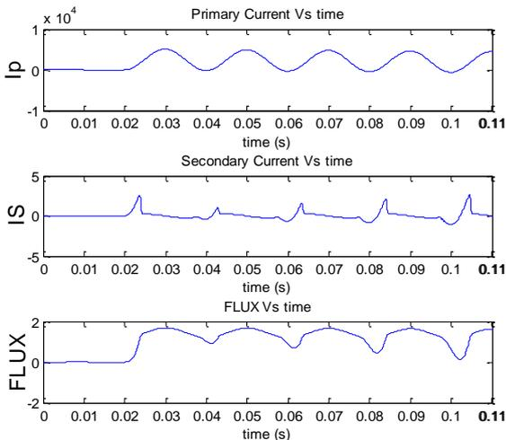
Figure13 Simulink Output At Asymmetry Current and Hysteresis with High Burden For Primary Current, Secondary Current and Flux .
