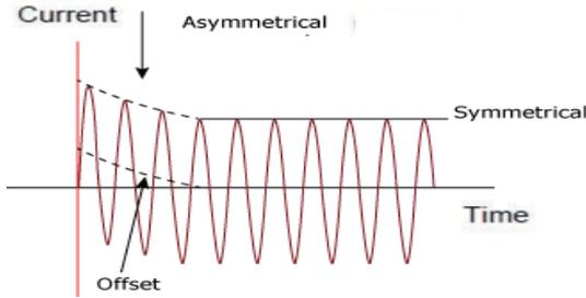
Figure 3 Fault Current with AC and DC Component Wave Form
