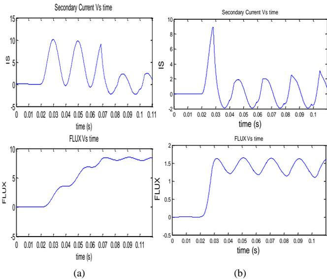
Figure (9) Simulink Output a) Without Hysteresis. b) with Hysteresis For Secondary Current and Flux.
