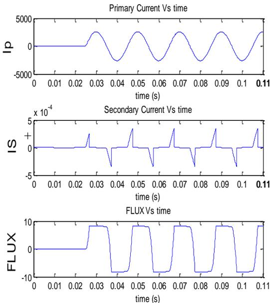
Figure 18 Simulink Output At Overvoltage for Primary Current, Secondary Current and Flux.
