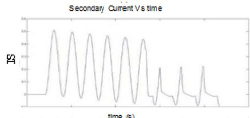
Fig 14 The Secondary Current when the X\R ratio = 0.628
