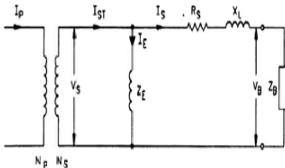
Figure 1Equivalent Circuit of CT
