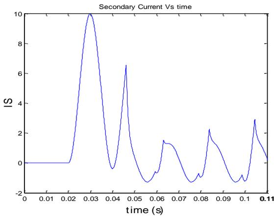
Fig 17 The Secondary Current When the CT ratio 2500:5
