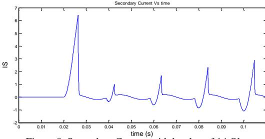
Figure 8 Secondary Current with burden of 14 Ohm
