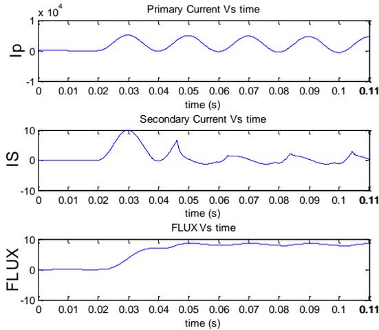
Figure 12 Simulink Output At Asymmetry Current Primary Current, Secondary Current and Flux.
