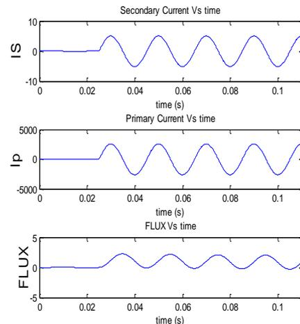
Figure 11 Simulink Output At No Asymmetry Current For Primary Current, Secondary Current and Flux .
