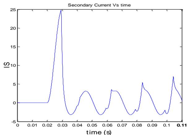
Fig 16 The Secondary Current When the .CT ratio 200:1
