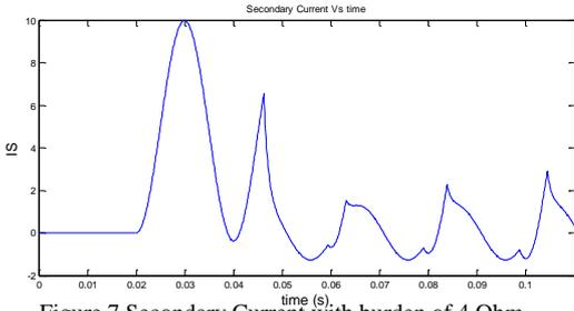
Figure 7 Secondary Current with burden of 4 Ohm,
