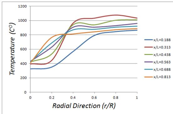
Fig 5 Temperature distribution in radial direction in the combustion chamber, for case (B) (Secondary Air inlet from front).
