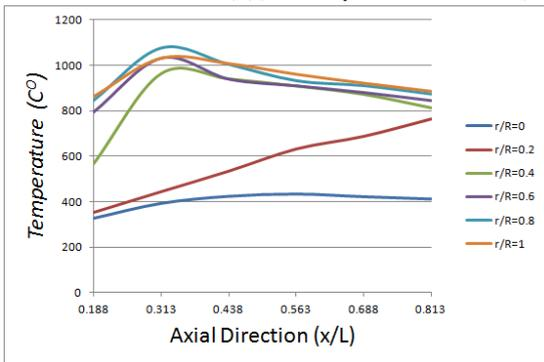
Fig 7 Temperature distribution in axial direction in the combustion chamber, for case (B) (Secondary Air inlet from front).
