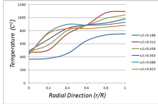
Fig 1 Temperature distribution in Radial direction in the combustion chamber, for case (A) (Secondary Air inlet from front).
