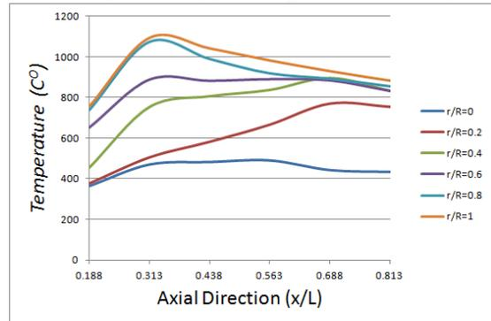
Fig 3 Temperature distribution in axial direction in the combustion chamber, for case (A) (Secondary Air inlet from front).
