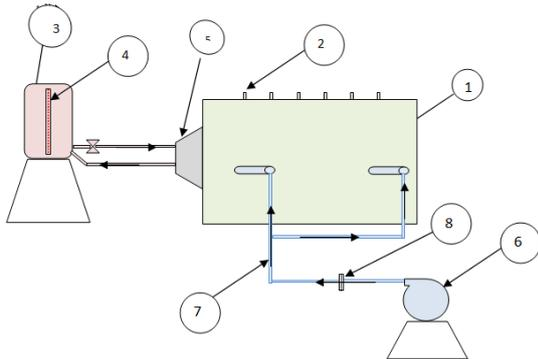
1-combustor. 2-measuring holes. 3-fuel tank. 4-fuel level indicator. 5-burning unit. 6-air blower 7-secondary air line 8-orifice meter
