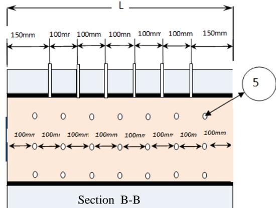
Fig 3 Arrangements and cases details of the secondary air entry.
