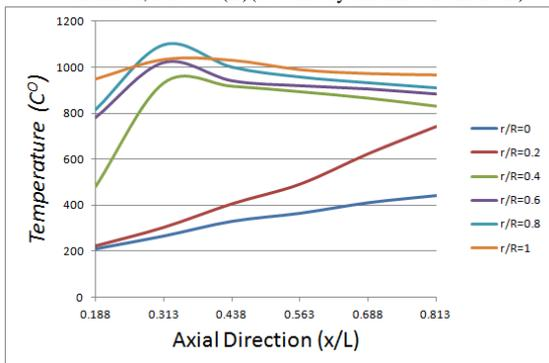
Fig 8. Temperature distribution in axial direction in the combustion chamber, for case (B) (Secondary Air inlet from back).
