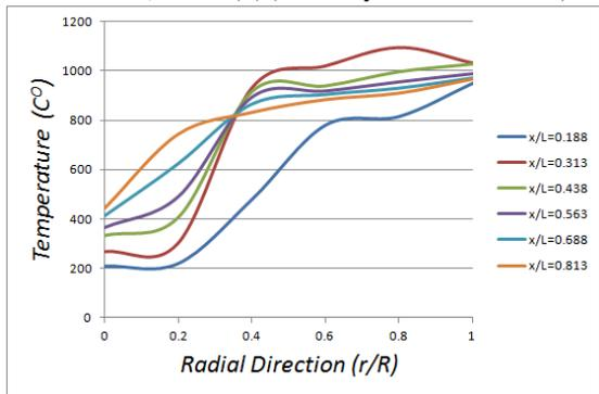
Fig 6 Temperature distribution in radial direction in the combustion chamber, for case (B) (Secondary Air inlet from back).
