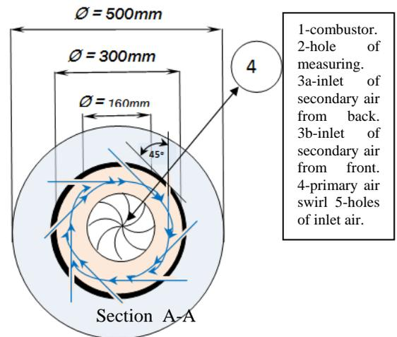
1-combustor. 2-hole of measuring. 3a-inlet of secondary air from back. 3b-inlet of secondary air from front. 4-primary air swirl 5-holes of inlet air.
