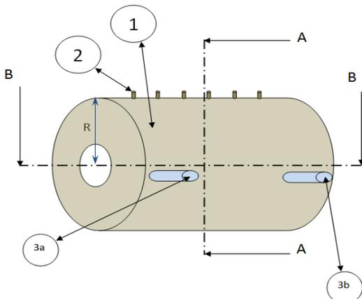
Fig 2 Details of the combustor.
