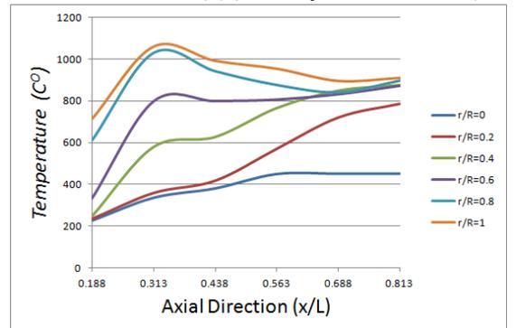
Fig 4 Temperature distribution in axial direction in the combustion chamber, for case(A) (Secondary Air inlet from back).
