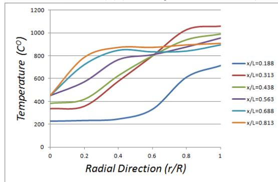
Fig 2 Temperature distribution in Radial direction in the combustion chamber, for case(A) (Secondary Air inlet from back).
