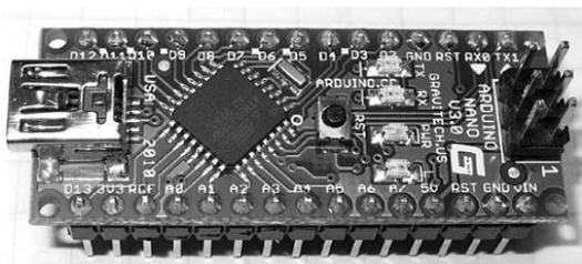
Figure 5. Arduino NANO board.
