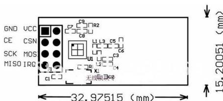
Figure 6. The nRF24L01 RF Module
