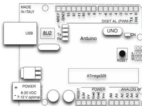
Figure 4. Arduino UNO board.
