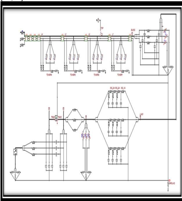
Figure 1. Shows the structure of 400kv studied system
