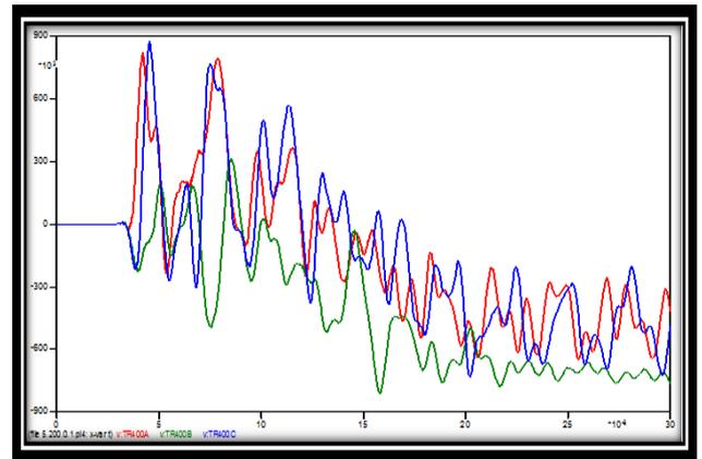
Figure 6. The inside voltage of the transformer when distance 10m of lightning current 260kA
