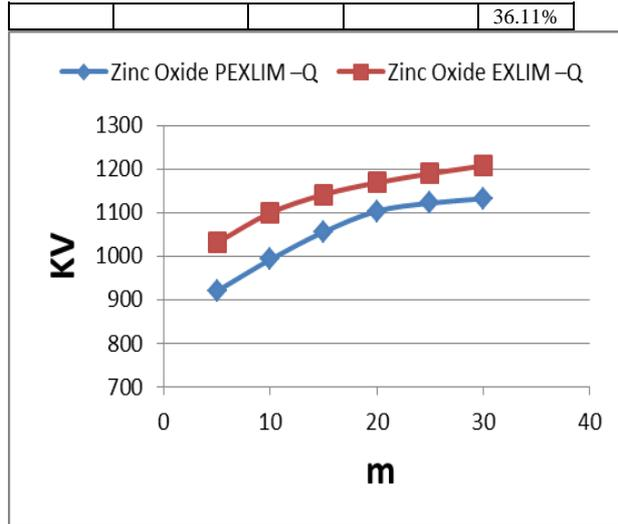
Figure 7. Effect of the arrester distance on inside voltage of transformer when be 260KA lightning current.
