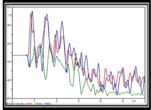
Figure 5 . The inside voltage of the transformer when distance 5m of lightning current 260kA
