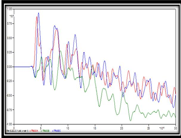
Figure 4. The inside voltage of the transformer when distance 10m of lightning current 260kA
