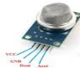
Fig 9: Gas Sensor(MQ2)
