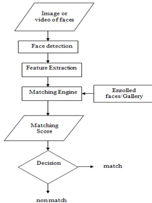
Fig 2: The basic flow of a recognition system
