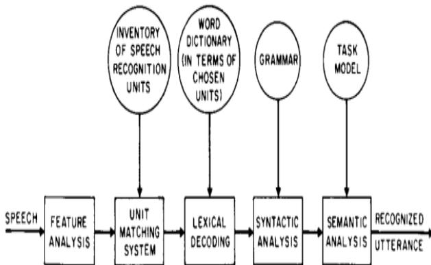
Fig 3: The block diagram of a speech recognizer
