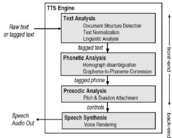
Fig 5: Block diagram of a general TTS
