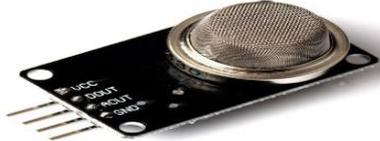
Fig 10: Gas Sensor(MQ135)
