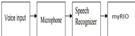
Fig 4: Block diagram for the SRS functioning integrated with Myrio.
